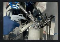
Using the trigger clamp, keep spray gun trigger in open position. Close auto clean compartment door or lid and set timer to 2-3 minutes.
